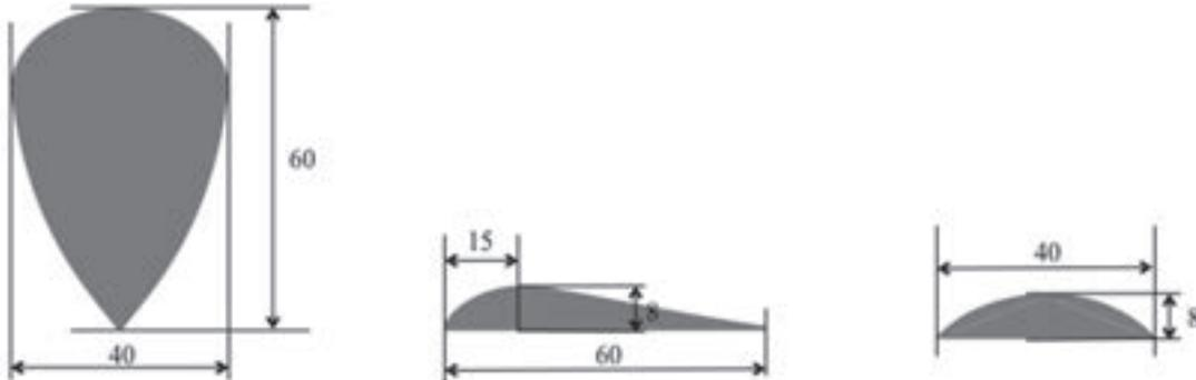
Figure 1. Dimensions of the metatarsal pad (unit: mm)
