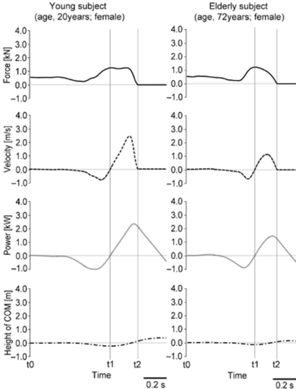
Figure 1. Time series of the force, velocity, power, and the height of the COM in a young (left) and an elderly (right) subject while they performed a CMJ. t0: the motion was initiated, t1: the COM was at the lowest point, and t2: the subject lost ground contact.
