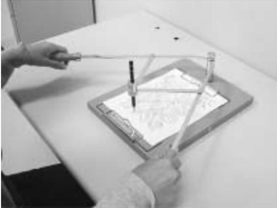
Fig. 1. Resonance test in general aptitude test for profession to measure the amount of cooperative motion.
