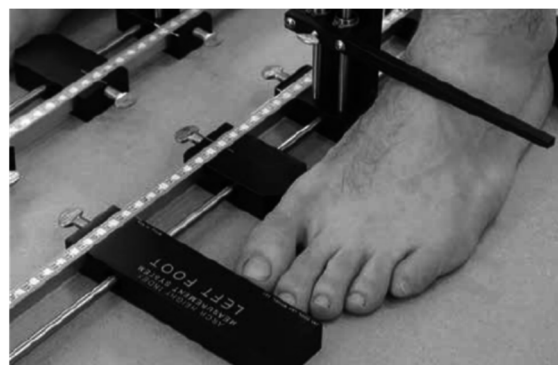
図1. Arch height index measurement system
