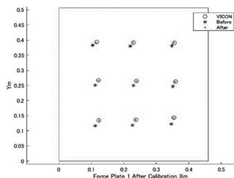
Fig. 2. Position of COP<sub>v</sub> and COP<sub>f</sub> data of the force plate 1 after calibration.
