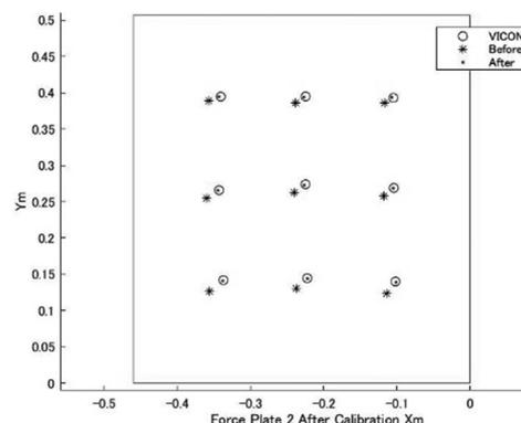
Fig. 3. Position of COP<sub>v</sub> and COP<sub>f</sub> data of the force plate 2 after calibration.
