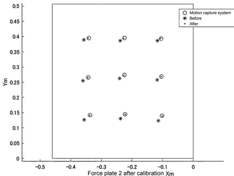
Figure 6. Position of COP<sub>v</sub> and COP<sub>f</sub> data of the force platform 2 after calibration.
