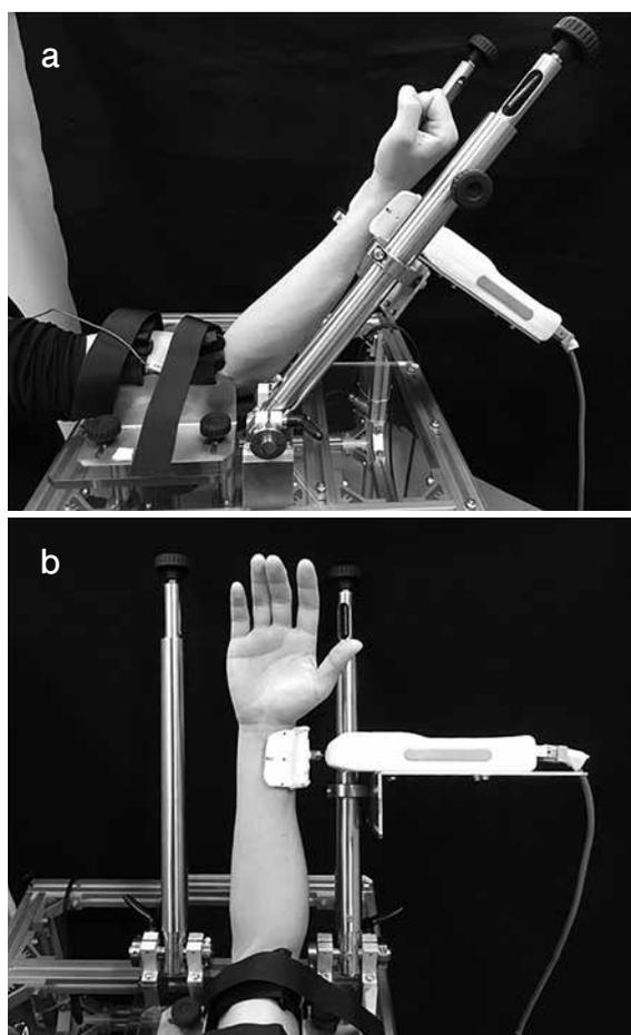
Figure 1. Measurement of EMGs of anconeus muscle and triceps brachii muscle. The movement tasks were isometric elbow extension (a) and valgus (b) movement, which were measured with an elbow torque measuring instrument.
