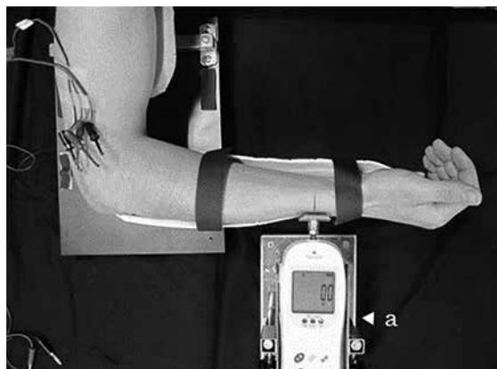
Figure 3. Measurement of elbow extension torque by electrical stimulation to anconeus muscle.
