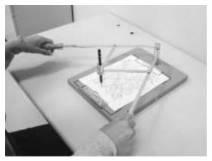
Fig. 1. Resonance test in general aptitude test for profession to measure the amount of cooperative motion.
