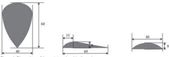
Figure 1. Dimensions of the metatarsal pad (unit: mm)
