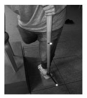
Fig. 1. Subject applying weight vertically on the force platform
