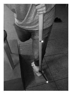
Figure 3. Subject applying weight vertically on the force platform.
